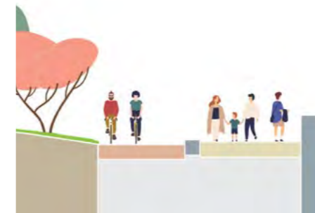
Cycle path - high colour contrast surfacing Widened footpath High contrast delineation
